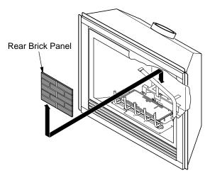
Figure 43 - Installing Rear Brick Panel
